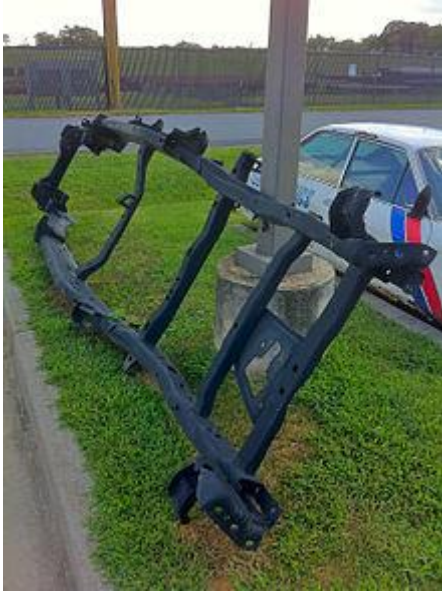
A vehicle's bare ladder frame
